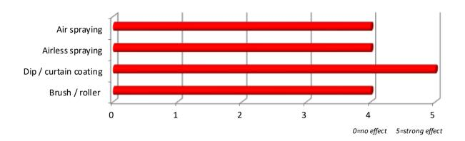
**UNIQ** FOAM 150 S is a strong defoamer can be used for all solvent borne coating systems, especially suitable for solvent free epoxy and solvent free UV system. The additive has an immediate foam-destroying effect with very strong deaeration and does not have influence on the intercoat adhesion.
